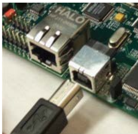
Figure 4-4: Connect the USB Type B Connector to the Starter Kit Board Connector
