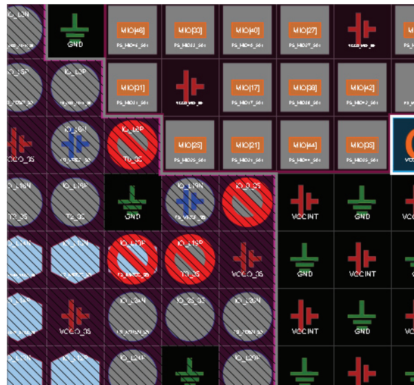
Figure 8-18: Setting Prohibits on Package Pins
