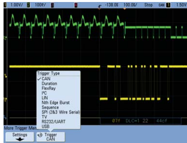
Trigger on and decode CAN serial packets.
