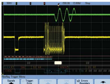
See mixed signal measurements in a FlexRay system using an MSO.
