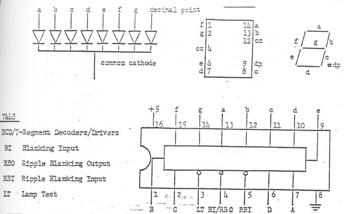
NCTE: Any output can be directly \_\_\_\_\_\_\_ connected to an LED since a dropping resistor is included in the output circuit.
