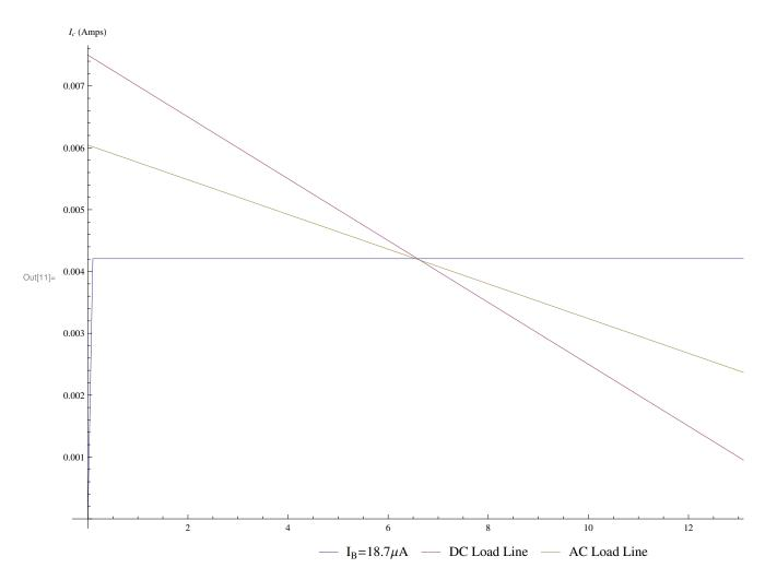
As you can see, the circuit is limited by saturation, as the maximum  $I_c$  is around 6 mA. This corresponds to an AC current component of about 2 mA on the collector, or 8  $\mu$ A on the base.
